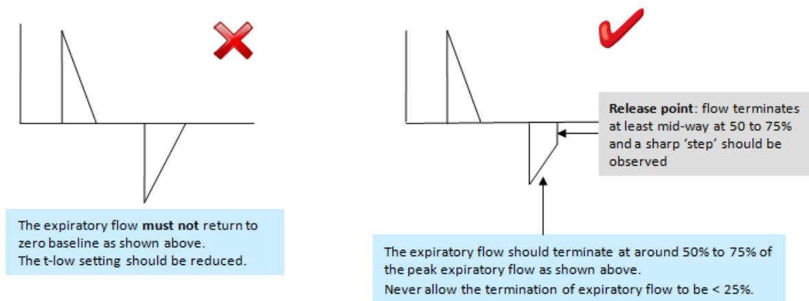
If the release point is at 75% **and** PaCO<sub>2</sub> is too high, consider increasing the t-low – but **only slow changes** are recommended, in increments of 0.05 to 0.1 seconds
